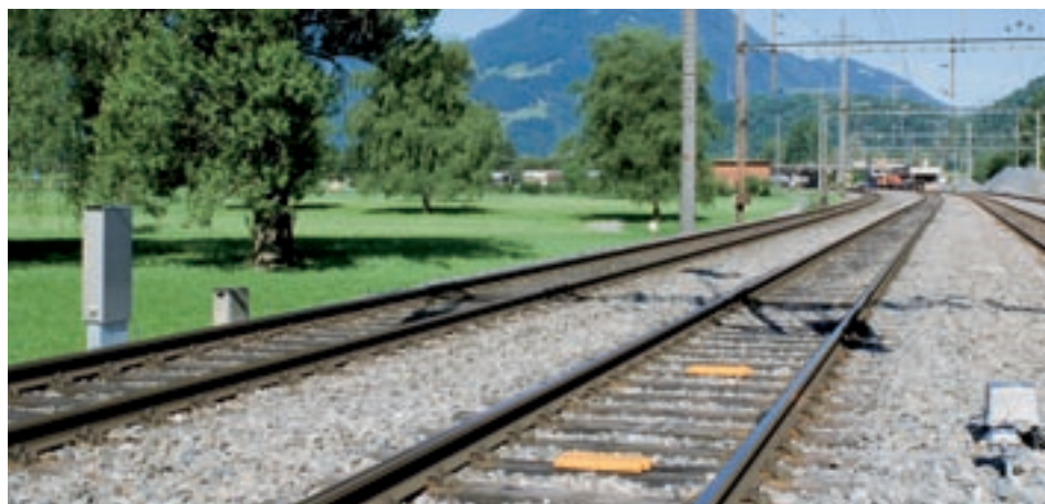
Transmission point with Trainguard Eurobalises S21
